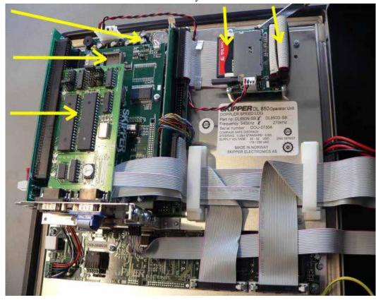
Parts list for DL850 DOU CPU6753, Compact flash and Disk-On-Chip.
